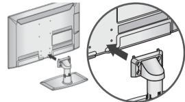
Fix the 4 bolts securely using the holes in the back of the TV.
