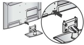
Assemble the parts of the Stand Rear Cover with the TV.
