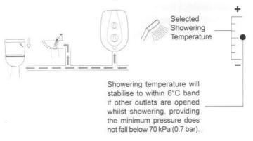
Water inlet pressure fluctuations due to other draw offs (e.g. flushing toilet) will cause the showering temperature to increase.
