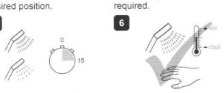
Allow 10 - 15 secs for any Check water temperature temperature adjustments before entering shower. to stabilise and reach the
