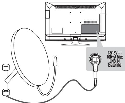
Connect the TV to a satellite dish to a satellite socket with a satellite RF cable (75 Ω).
