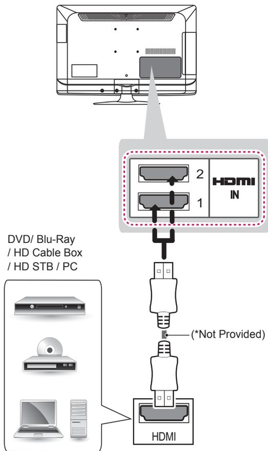
Transmits the digital video and audio signals from an external device to the TV. Connect the external device and the TV with the HDMI cable as shown in the following illustration. Choose any HDMI input port to connect. It does not matter which port you use.
