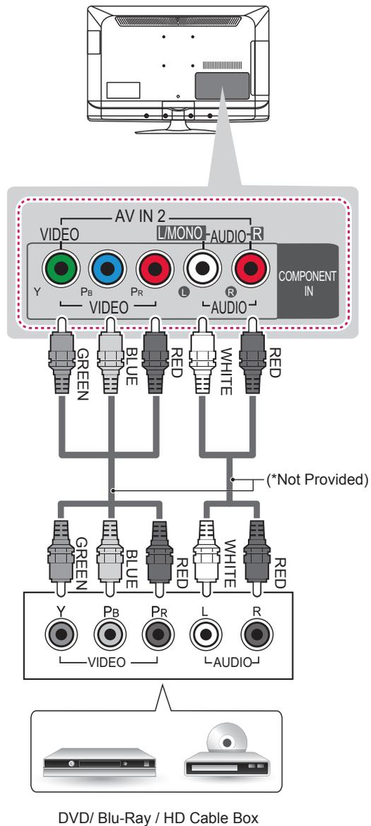
Transmits analog video and audio signals from an external device to the TV. Connect the external device and the TV with a component cable as shown.
