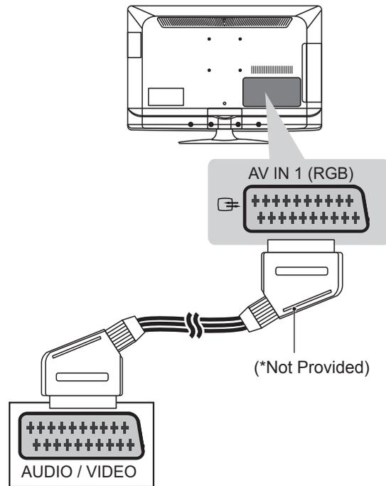
Transmits the video and audio signals from an external device to the TV set. Connect the external device and the TV set with the euro scart cable as shown. To display images by using progressive scan, make sure to use the euro scart cable.
