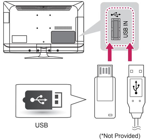
Connect a USB storage device such as a USB flash memory, external hard drive, or a USB memory card reader to the TV and access the My media menu to use various multimedia files.
