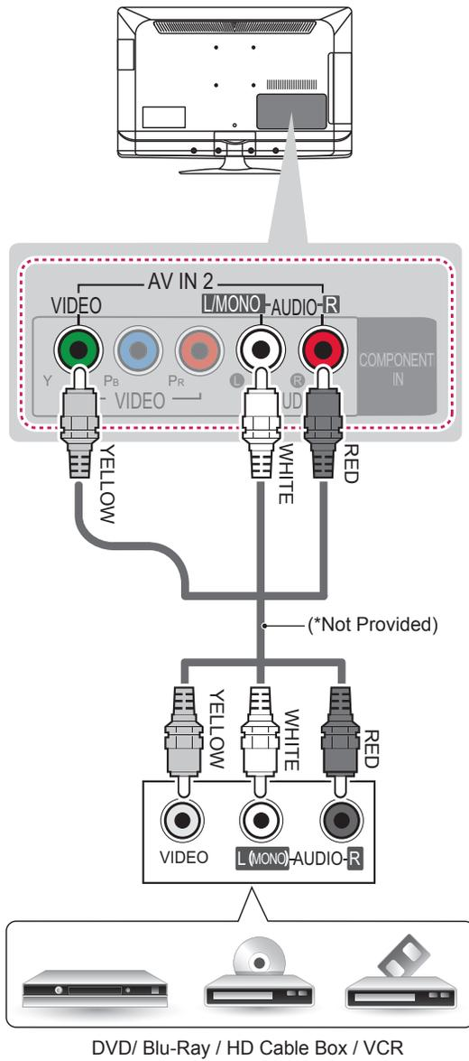
Transmits analog video and audio signals from an external device to the TV. Connect the external device and the TV with the composite cable as shown.
