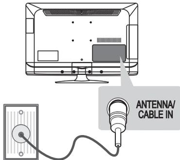
Connect the TV to a wall antenna socket with an RF cable (75 Ω).
